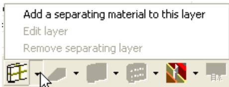
This layer allows the consideration of layers bridged by metal structures, which is excluded from the scope of BS EN ISO 6946. Such situations are typical for steel frame constructions. The calculation rule used is described in BRE, Digest 465. The calculation is similar to that used when calculating other inhomogeneous layers.
